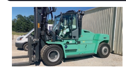
2023 Mitsubishi FD 160L12P ID# 23PN2367 197"/130"/66" Triplex Mast - 96" Forks S/S F/P Diesel Base Capacity: 36,000 lbs. @ 48" LC
