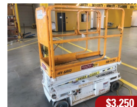
Hybrid HB1430 Scissor Lift 24V DC Scissor Lift, 30" wide, 14' platform height. 2014 - 191 Hrs. - #1418R2005
