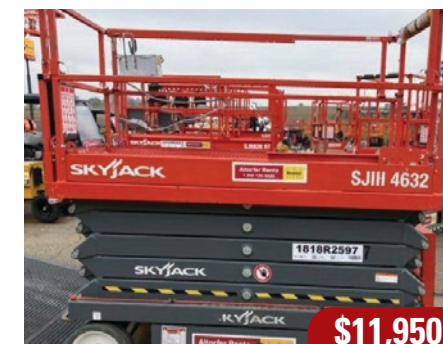
Skyjack 4632 Scissor Lift 24V DC Scissor Lift, 46" wide, 32' platform height. 2018 - 256 Hrs. - #1818R2597
