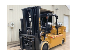
2024 Lowry L300XDS ID# 23CN2114 144"/103"/48" Triplex Mast - 96" Forks S/S F/P - 2 LP Tanks Base Capacity: 30,000 lbs. @ 24" LC
