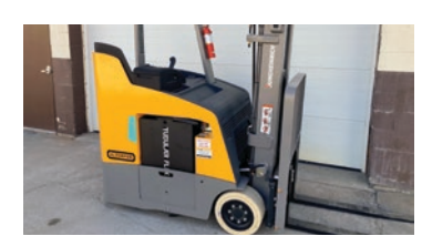
2023 Jungheinrich ETG318 ID# 23EN1324 188"/83"/35" Triplex Mast - 48" Forks - Dock Stocker S/S F/P - 36V Battery Base Capacity: 4,000 lbs. @ 24" LC
