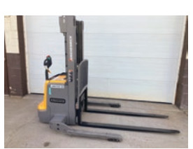
2023 Jungheinrich EJC16A ID# 23EN1329 180"/80"/57" Triplex Mast - Heavy Duty Straddle Stacker 24V Battery with On Board Charger Base Capacity: 3,500 lbs. @ 24" LC
