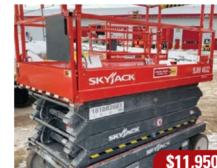
Skyjack 4632 Scissor Lift 24V DC Scissor Lift, 46" wide, 32' platform height. 2018 - 246 Hrs. - #1818R2693
