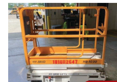
Hybrid HB1030 Scissor Lift 24V DC Scissor Lift, 30" wide, 10' platform height. 2018 - 119 Hrs. - #1818R2647
