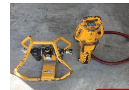
Rhino PD-55 Post Driver Pneumatic Powered, Post Driver, 3-7/8" id chuck. 2020 - Hrs. N/A - #2021R670
