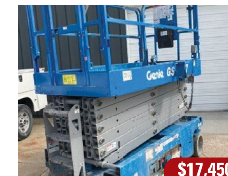
Genie GS4047 Scissor Lift 24V DC Scissor Lift, 47" wide, 40' platform height. 2016 - 259 Hrs. - #1618R2194
