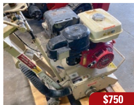
Edco CPM89H Scarifier Gas powered, walk behind scarifier, 8" working width. 2008 – Hrs. N/A – #1413U4
