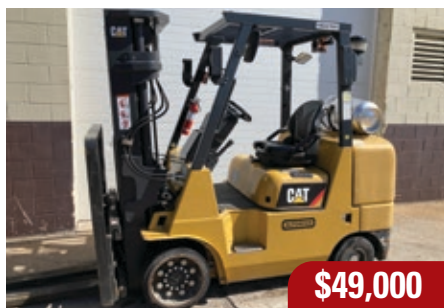
2019 Caterpillar GC40K-LE ID# 19CN1924 183"/87"/39.5" Triplex Mast 72" Forks – S/S F/P – LP Tank Base Capacity: 8,000 lbs. @ 24" LC
