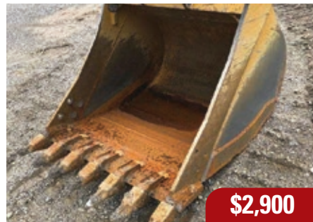
Cat 42" General Duty Bucket 315 excavator mount, .84 cubic yard capacity 2019 – #192RA1391
