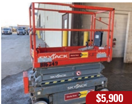
Skyjack 3219 Scissor Lift 24V DC Scissor Lift, 32" wide, 19' platform height. 2014 – 189 Hrs. – #B16349
