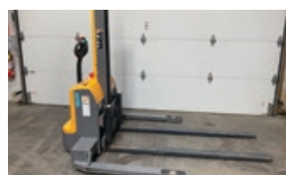
2022 Jungheinrich EMCB10 Walkie Straddle Stacker ID# 22EN1328 60.5"/77.5"/29.5" Mast, 48" Forks – 24V On Board Charger Base Capacity: 2200 lbs. @ 24" LC
