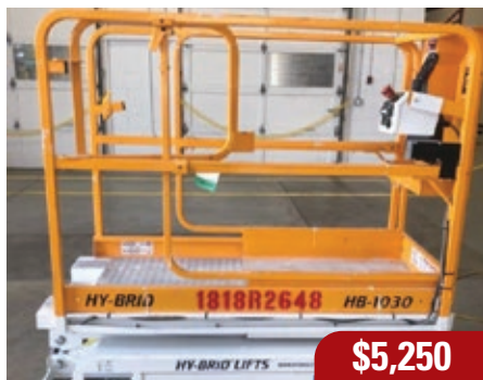
Hybrid HB1030 Scissor Lift 24V DC Scissor Lift, 30" wide, 10' platform height. 2018 – 192 Hrs. – #1818R2648
