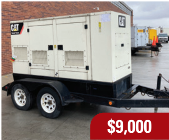
2009 XQ60 F0627 Cat Tier 3 C4.4 Engine Sound Attenuated Enclosure Maintained by Cat Cert. Technicians since new 26,333 Hrs.
