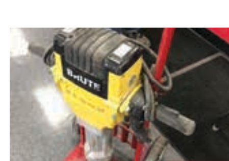
Bosch Model BH2760VCB 110V DC, 35 ft/lbs impact energy, 1-1/8" chuck 2018 - Hrs. NA - #1815R80
