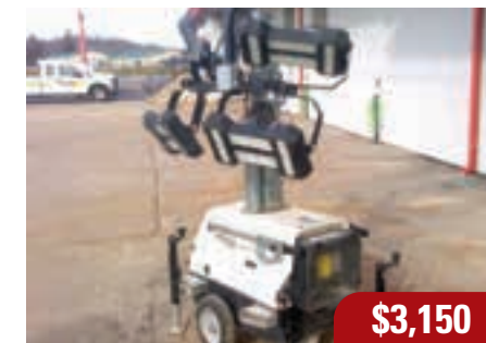
Generac PLT 240 LED Light Tower 110V DC, 16' vertical mast 4 240W LED lights 2017 - Hrs. NA - #1719R1605
