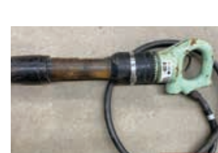
Sullair MRB-8 Rivet Buster Air consumption 44cfm, 1140 blows/minute 2021 - Hrs. NA - #2021R710
