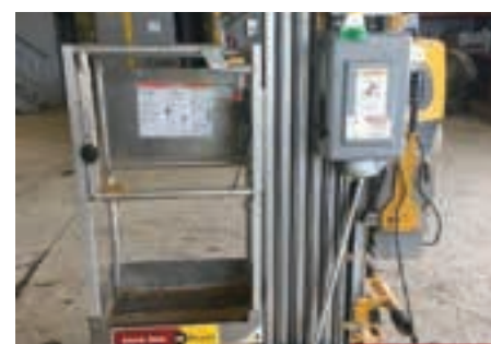
Genie AWP-30 Single Man Lift 12V DC, 29' 6" platform height 2015 - Hrs. NA - #B07445
