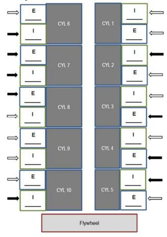
Use a 17mm wrench to loosen the nut around the lash adjuster you are going to set. Use a screwdriver to set the valve lash adjuster so that the feeler gauge of your desired thickness fits into the gap between the rocker arm and the valve tip. The gauge should fit snugly, but should still slide in and out – don't clamp the rocker arm onto the feeler gauge.
