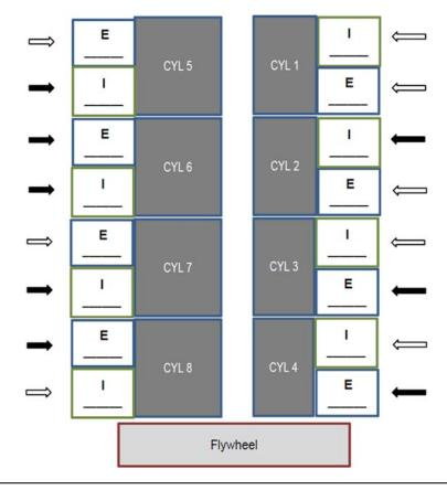
Use a 17mm wrench to loosen the nut around the lash adjuster you are going to set. Use a screwdriver to set the valve lash adjuster so that the feeler gauge of your desired thickness fits into the gap between the rocker arm and the valve tip. The gauge should fit snugly, but should still slide in and out – don't clamp the rocker arm onto the feeler gauge.
