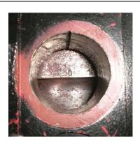
Another way to verify that the camshaft is in the correct position is to watch the rockers on cylinder #1 as the crankshaft is rotated. If the rockers are moving as the crankshaft approaches TDC #1, the crank will need to be rotated 360 degrees to set the engine for timing. If the rockers on cylinder #1 do not move as you approach TDC #1, the timing is correct and you may begin checking valve lash.
