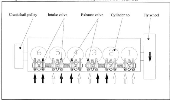
Use a 17mm wrench to loosen the nut around the lash adjuster you are going to set. Use a screwdriver to set the valve lash adjuster so that the feeler gauge of your desired thickness fits into the gap between the rocker arm and the valve tip. The gauge should fit snugly, but should still slide in and out – don't clamp the rocker arm onto the feeler gauge.
