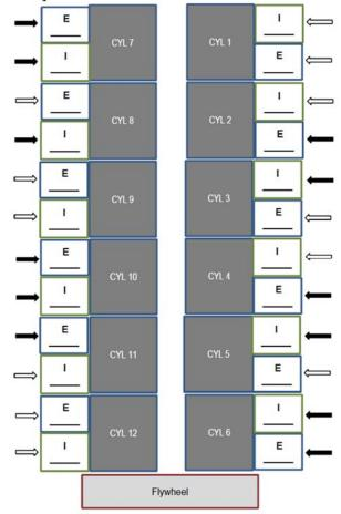
Use a 17mm wrench to loosen the nut around the lash adjuster you are going to set. Use a screwdriver to set the valve lash adjuster so that the feeler gauge of your desired thickness fits into the gap between the rocker arm and the valve tip. The gauge should fit snugly, but should still slide in and out – don't clamp the rocker arm onto the feeler gauge.
