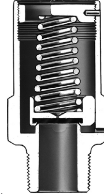
Figure 2. Sectional View of H200 Series Relief Valve
