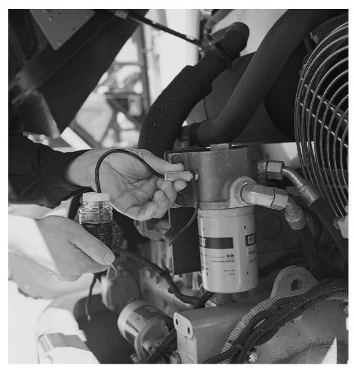
because they come from a consistent, known location where the fluid is well mixed and circulated. If the oil flow is slow at low idle, it may be necessary to have someone accelerate the engine to high idle while extracting the sample. Do not take your oil sample from the drain stream, because dirty oil from the bottom of the compartment will contaminate the sample. Likewise, never dip an oil sample from an oil container or pour a sample from a used filter.
